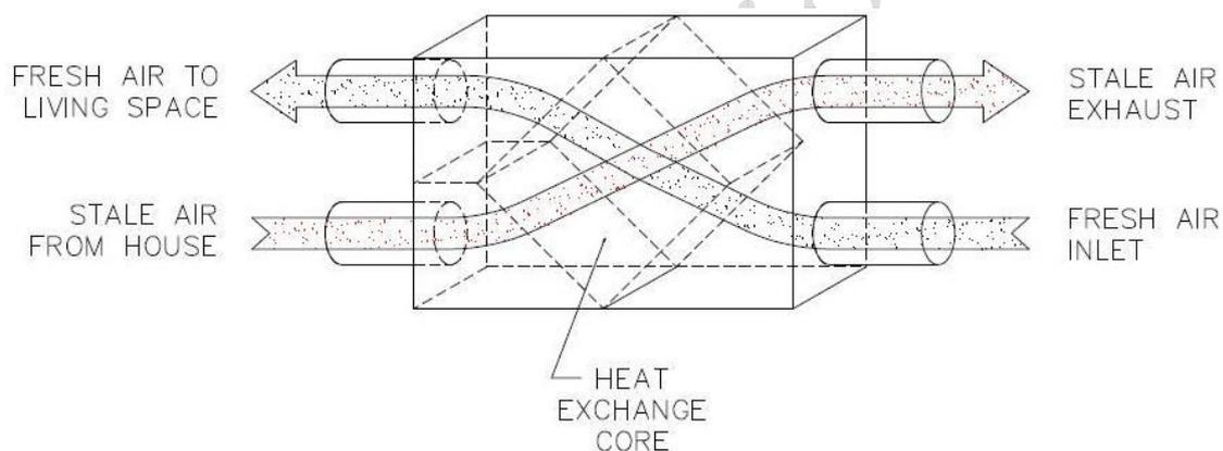
**A true Heat Recovery Ventilation system (HRV)** uses a metal heat exchanger (often aluminum). As the stale damp warm air from the home passes through the heat exchanger the moisture condenses and requires a drain to run the excess away.
